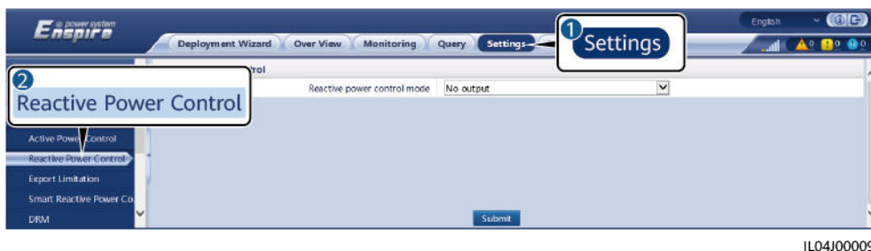
Figure 6-51 Reactive power control
