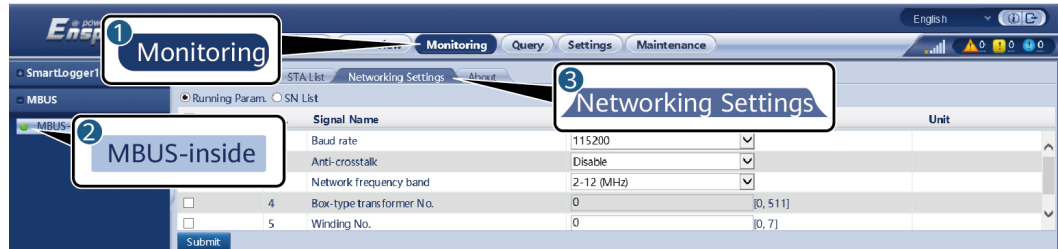
Figure 6-18 Setting the built-in MBUS networking
