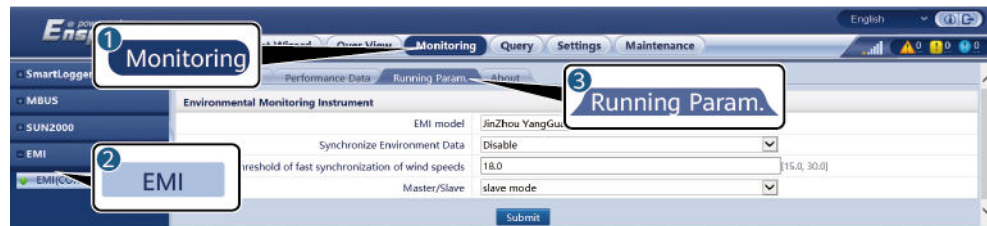
Figure 6-33 Setting running parameters
