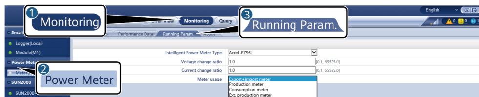
Figure 6-31 Setting power meter parameters
