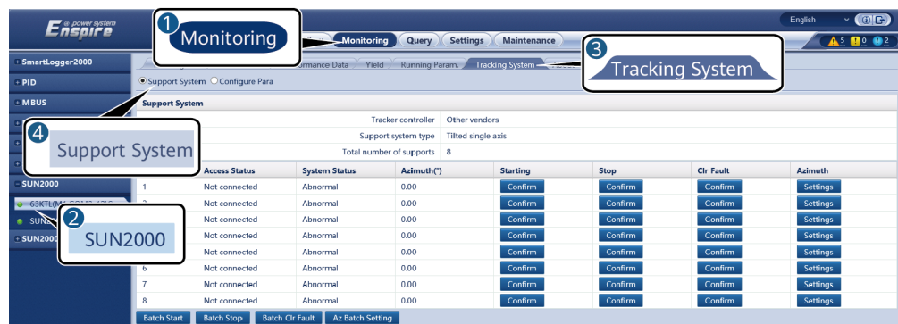
Figure 6-24 Support system (tracking system)
