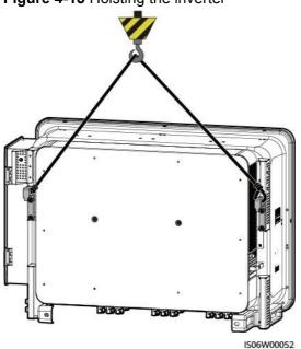
Figure 4-15 Hoisting the inverter
