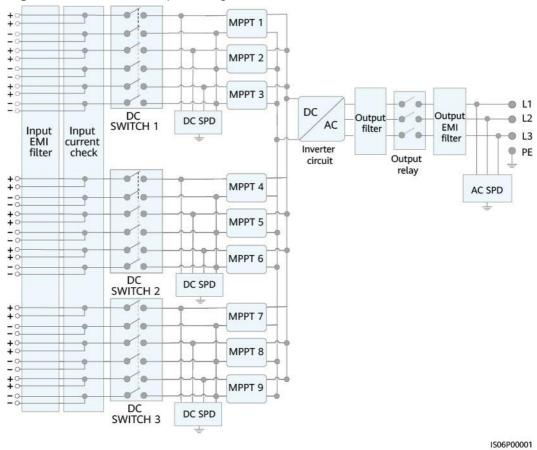
Figure 2-6 Inverter conceptual diagram
