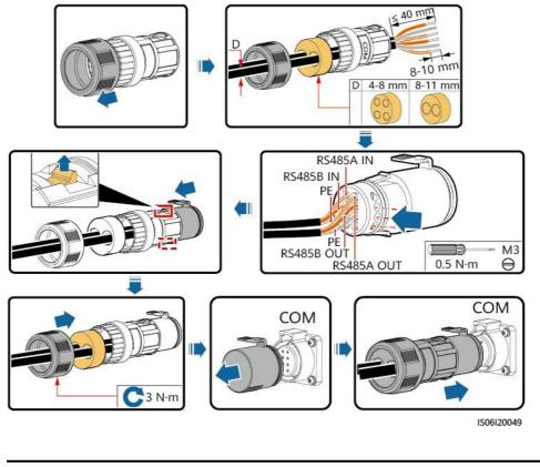
Figure 5-17 Cable connection (4-8 mm four-hole rubber plug)
