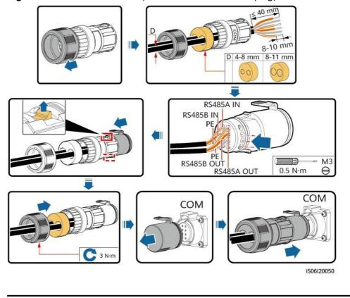
Figure 5-18 Cable connection (4-8 mm two-hole rubber plug)
