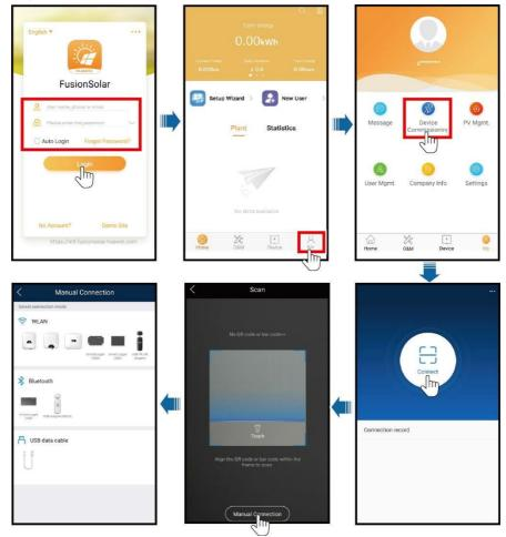
Figure 7-3 Selecting a connection mode (with network access)
