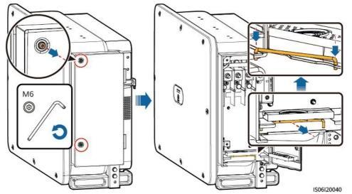
Figure 5-4 Opening the maintenance compartment door
