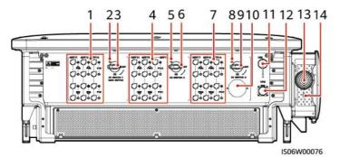
(1) DC input terminals (controlled by DC SWITCH 1)
