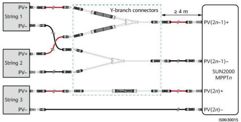
Figure 5-14 Connecting Y-branch connectors to the solar inverter
