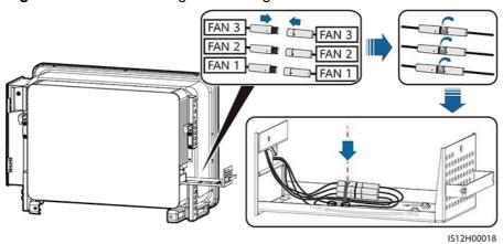
Figure 8-15 Reconnecting and binding the cables
